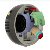
You can slide in the "Speaker & Switch Holder" into the "Middle Ring - Electronics Holder" The other two completed parts "Inner Slide" and "Auxiliary Switch" will be fitted into the "Dome Top" Inner parts completed
